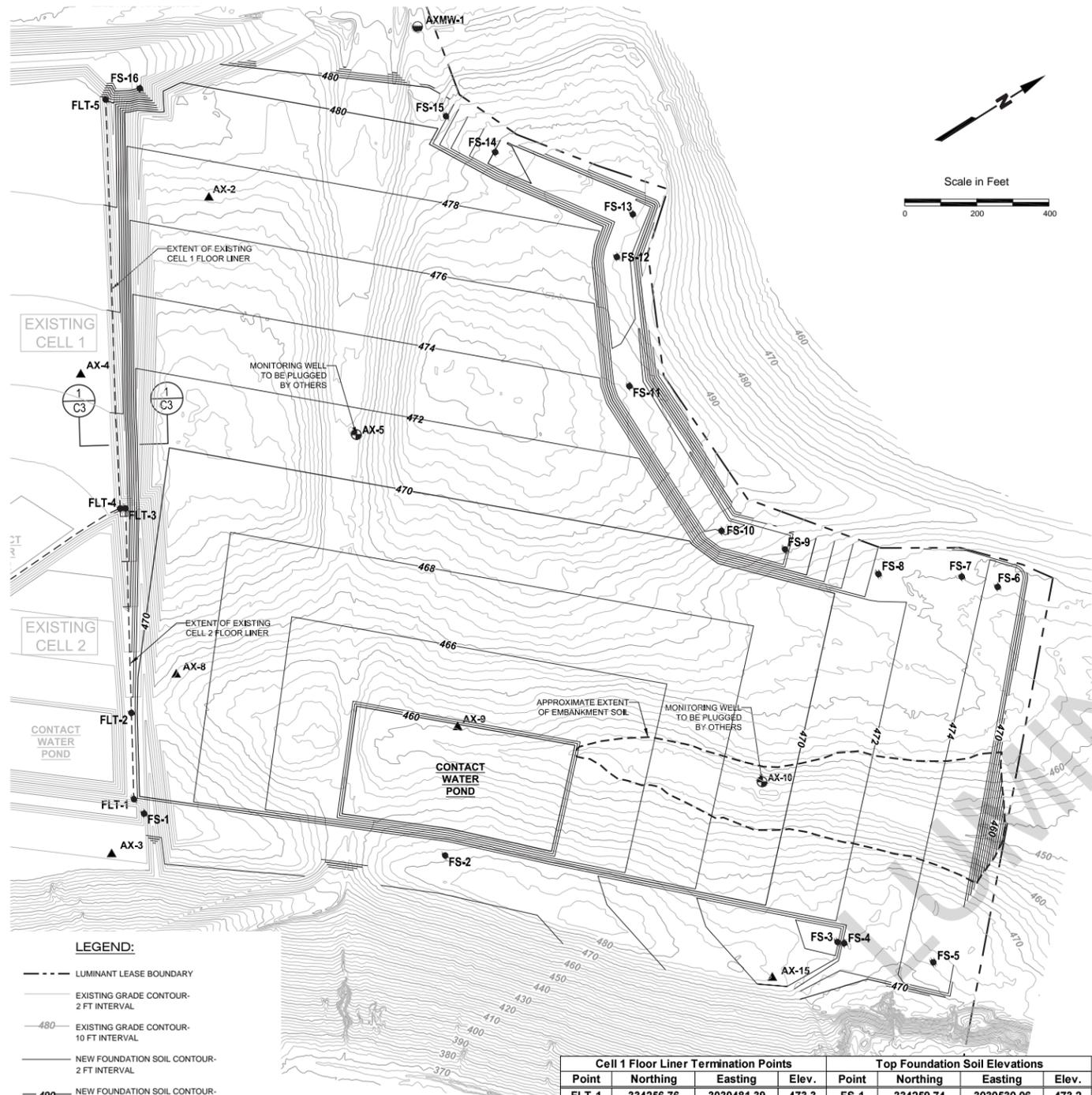
**CELL NO. 2A FOUNDATION SOIL PLAN**
