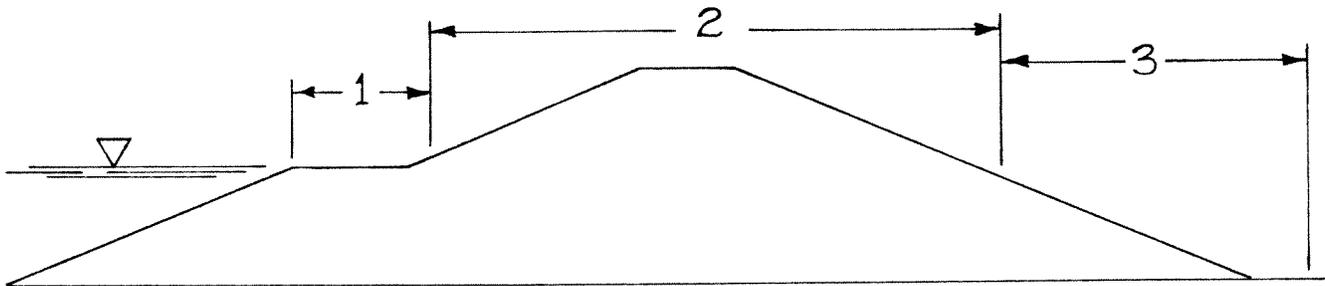
1. Waterline - Potential problems include slope damage from tree blowdown, visual masking of the structure that may hinder clear observation of a potential problem, tree root interception of spillway conduits, treetop interference with hydraulic performance of principal spillways and wave action scour due to obstructions.
