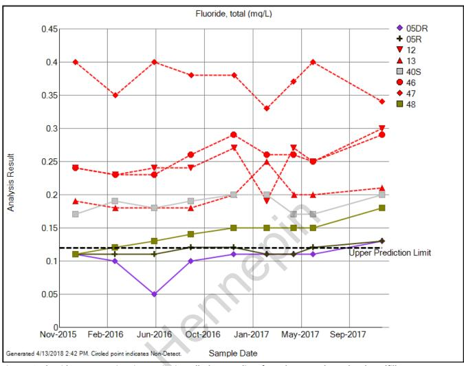
Figure 10. Fluoride concentration time-series in wells downgradient from the East Ash Pond and Landfill.
