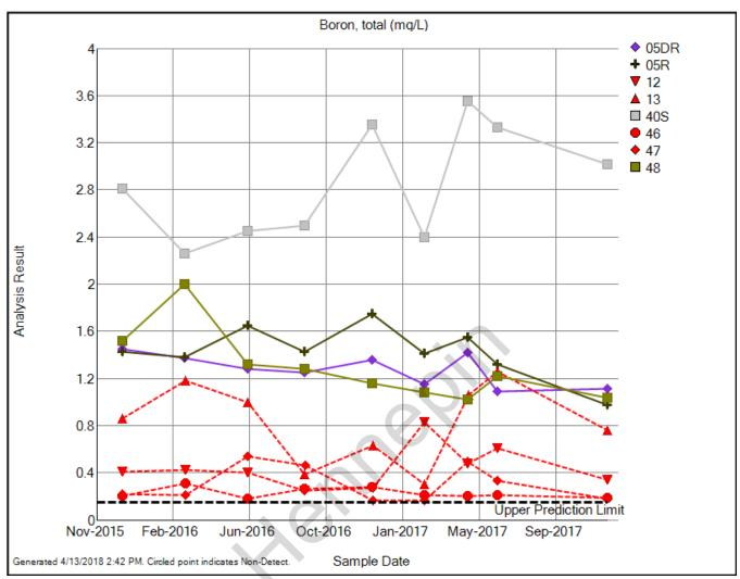
Figure 9. Boron concentration time-series in wells downgradient from the East Ash Pond and Landfill.
