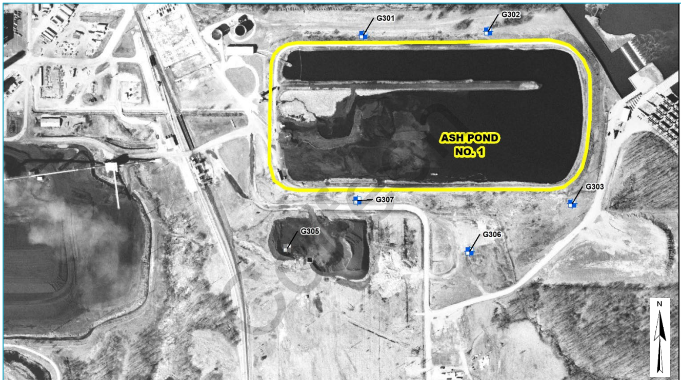
Figure 2. An aerial photograph from April 2005 2 shows potential coal storage near G307 and G306, and a mine shaft (black box) near G305. Groundwater generally flows from the southwest to the northeast across AP1.
