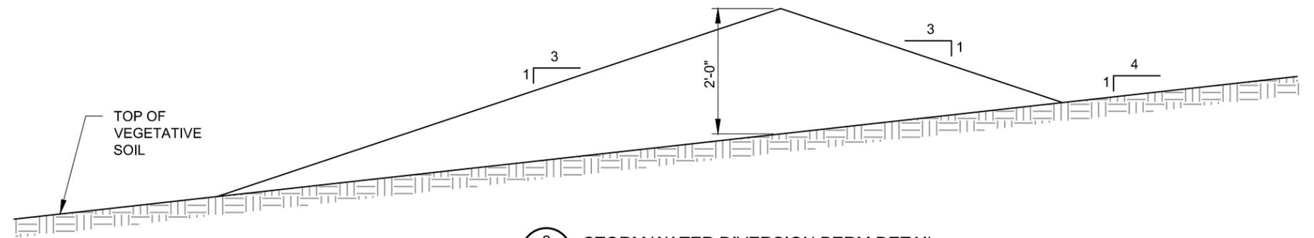
2 STORM WATER DIVERSION BERM DETAIL
