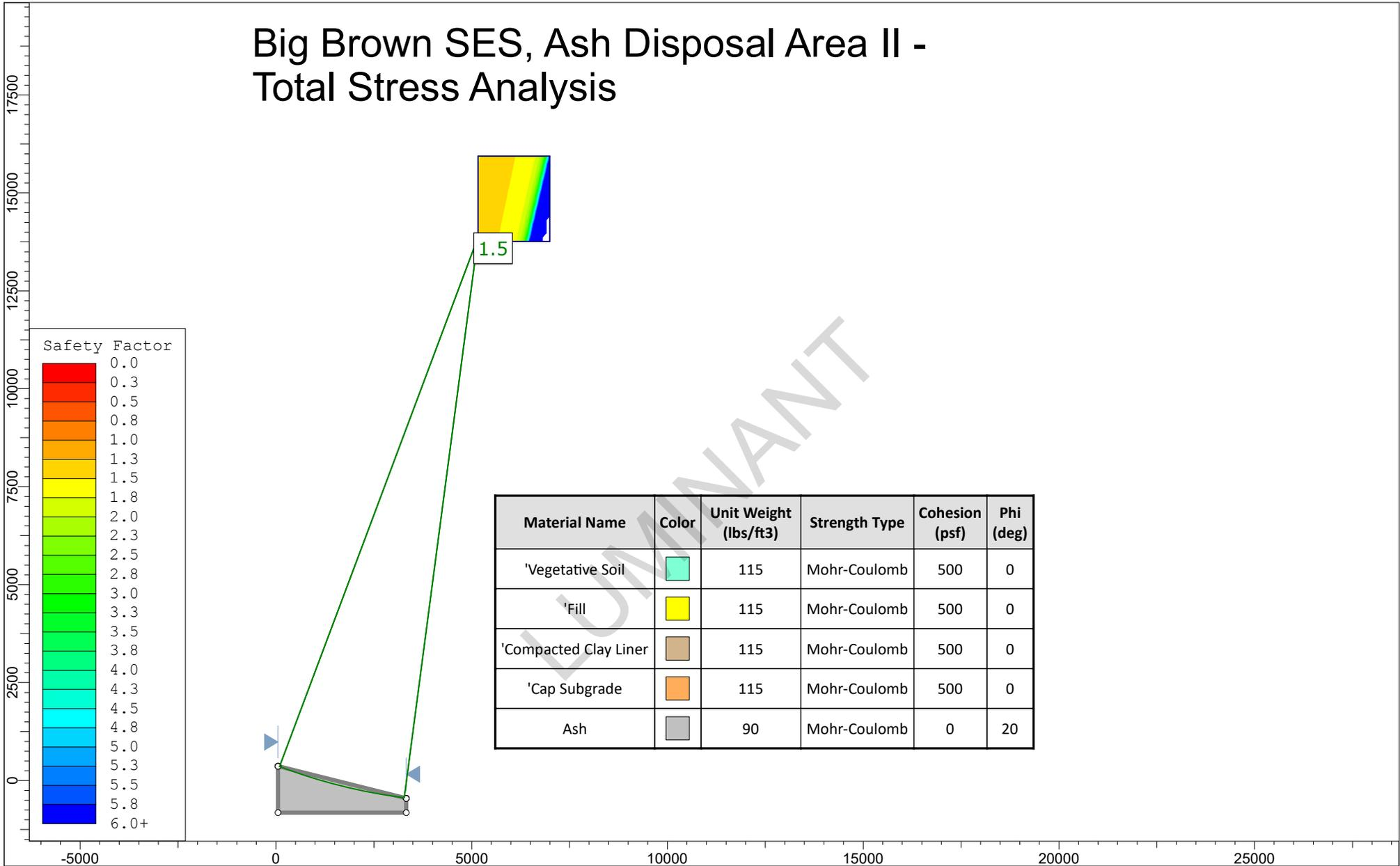
Veneer Cover Soil Analysis of Synthetic Cap System
