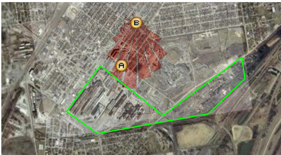
Figure 3-5. Results of an analysis of excess PM 2.5 concentrations at the Granite City monitoring site (Sprague, 2010a) 2 .
